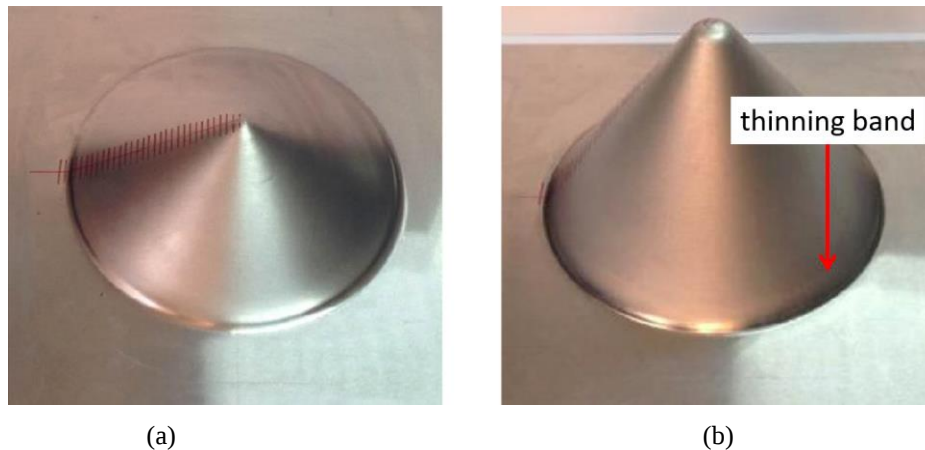
Fig. 4. MSPIF process application: (a) Cone after 1 o tool pass and (b) cone after 2 o tool pass [14]
