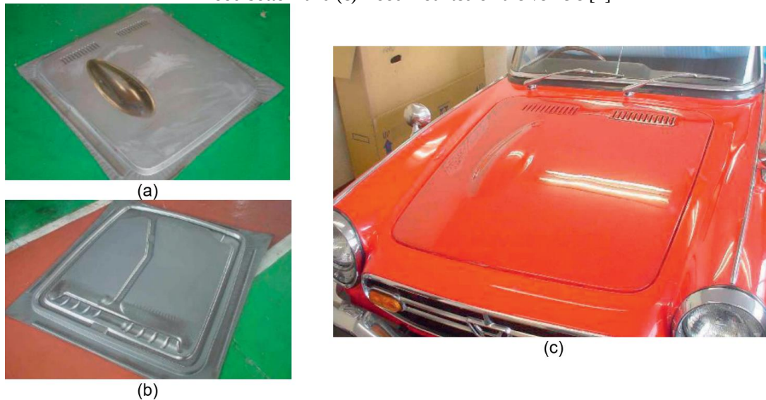
Fig. 7. Honda S800 hood manufactured with Incremental Sheet Forming: (a) Patterned hood top, (b) Hood bottom and (c) Hood mounted on the vehicle [1]
