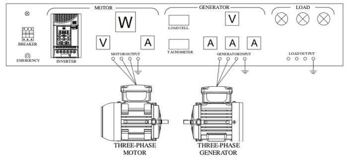
Figure 9 – Schematic drawings of the proposed bench.
