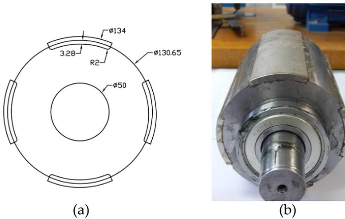
Figure 5 – Smooth pole rotor – (a) Schematic drawings – (b) rotor assembled [6]
