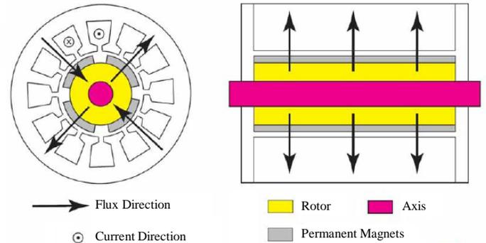
**Figure 1 – Radial flux machine [7]**
