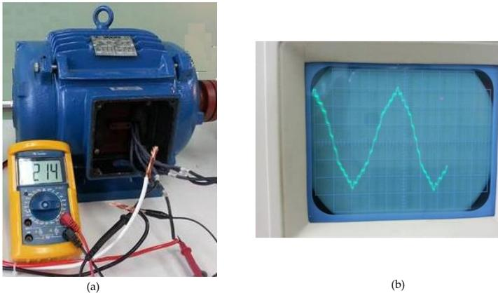
**Figure 12 – Generator test – (a) Voltage Reading – (b) Waveform [12]**
