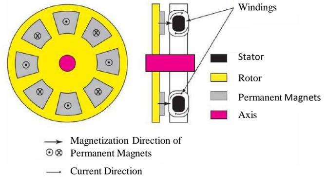
**Figure 2 – Axial flux machine [7]**
