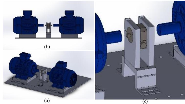
**Figure 7 – Schemes for tests of Rotatory Electric Machines – (a) Perspective view – (b) Front view – (c) Load cell detail**
