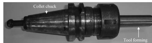
**Figure 1.** Tool forming mounted into collet chuck.
