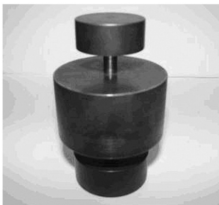
Fig. 2. Matrix to obtain the samples.
