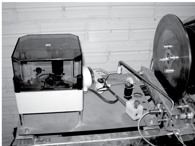
Figure 1. Braking system of Wind Energy Converter (WEC).
