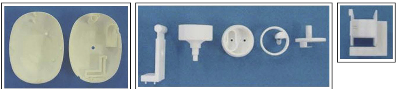
Fig. 10. Prototyped model-air compressor developed by LdSM.
