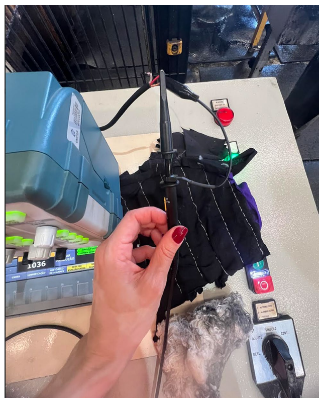
Fig. 6 RS485 connection to the oscilloscope
