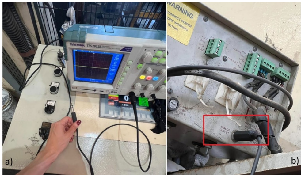
Fig. 7 (a) Analog cable connection to the oscilloscope; (b) verification of the analog output signal of the load cells
