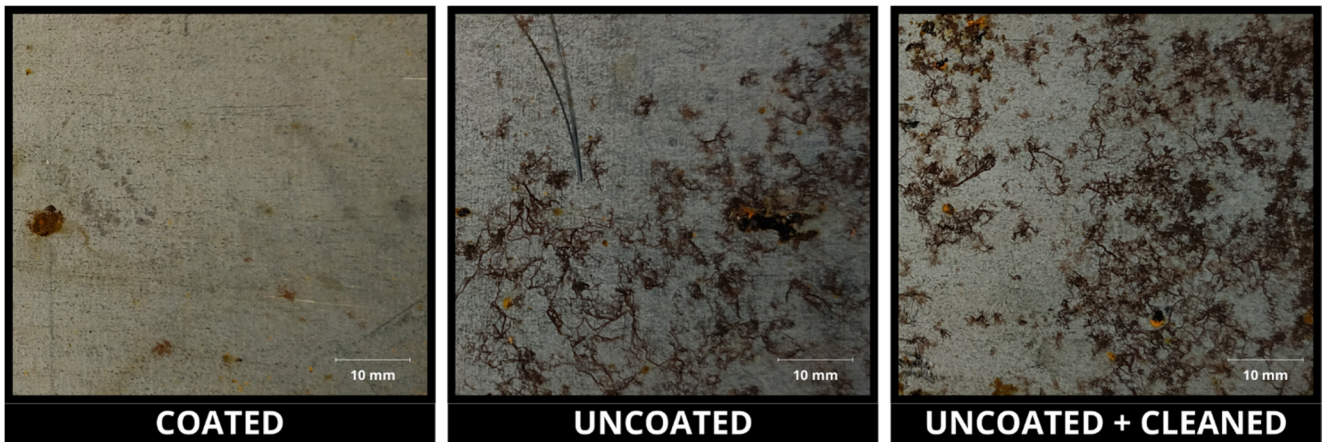
Fig. 10 Representative surface images of the three test conditions after 168 h of exposure in the saturated humid chamber
