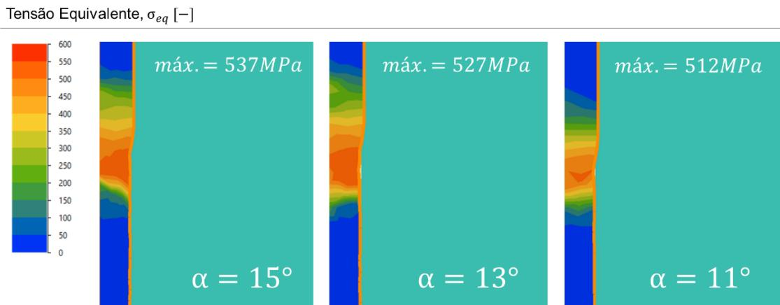
Figure 6 shows the equivalent stress distribution obtained numerically after the extrusion process. It was observed that, with the increase in the die angle, the equivalent stress in the work material also increases, indicating a direct relationship between the extrusion angle and the mechanical effort required by the process. Figure 7 demonstrates the variation of forces in the extrusion process, for the variations in the die entry angles.
