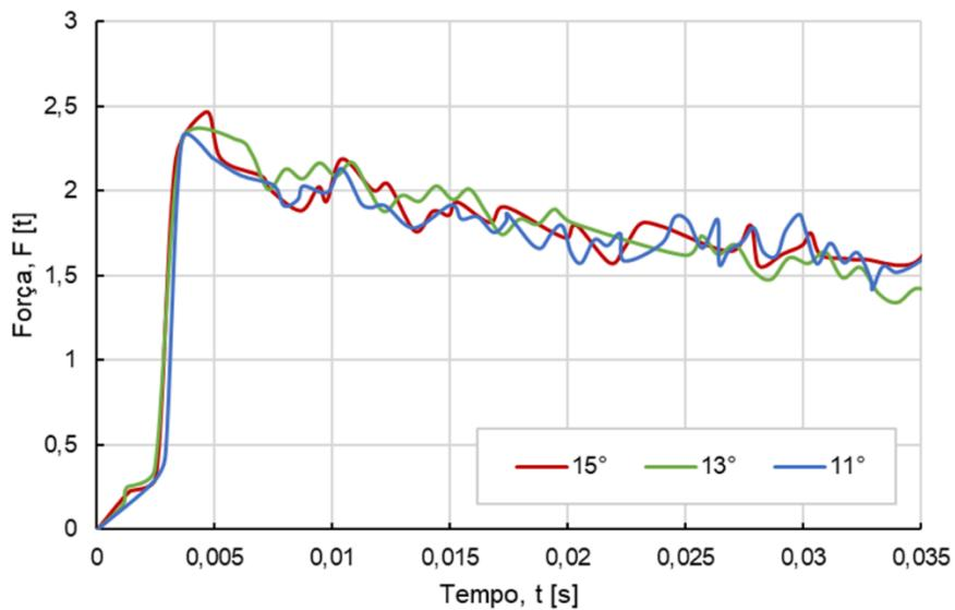
The numerical results obtained by finite elements demonstrated consistency with the analytical predictions, confirming that the forming force increases with the die angle. For the evaluated angles, the maximum simulated forces were 2.30 t for  $\alpha = 11^\circ$ , 2.35 t for  $\alpha = 13^\circ$  and
