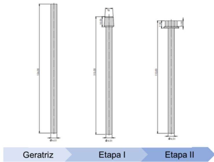
To increase efficiency in the use of raw materials and reduce production costs, a new manufacturing route was proposed (Figure 2). The initial stage, previously limited to simple pressing, now includes direct extrusion of the screw body. This additional material flow facilitates adequate filling during the final forming stage of the hexagonal head, also allowing the initial dimension of the generator to be reduced.
