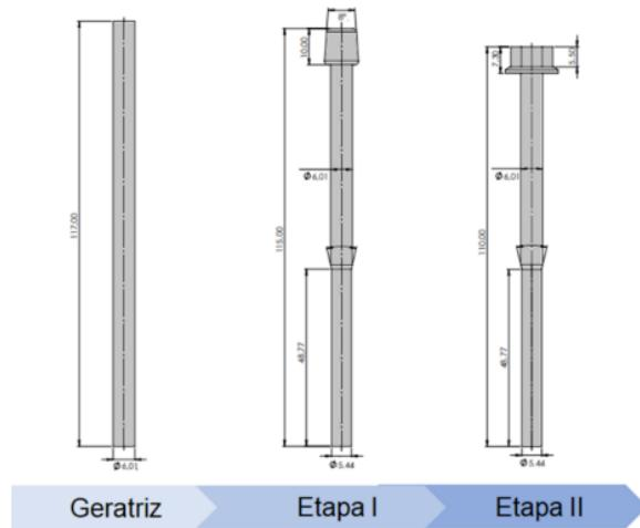
The development of this new forming stage requires a precise choice of the extrusion angle. This seeks to improve the efficiency of the process, reducing the force required for forging, energy consumption and wear on the tools used.
