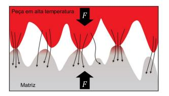
Equation 17 shows heat transfer at the interface between the blank and the matrix. The blank surface area in contact with the matrix (Abd1) is again considered.
