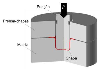
It is also assumed that the heat lost to the environment is negligible, since puncture and matrix temperatures are controlled by the cooling fluid over time. After the forming step, the blank is kept in the closed tool to allow cooling for about 15 to 25s (Steinbeiss, 2007).
