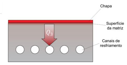
To determine the amount of heat transferred, conduction form factor analysis can be used (Ji, 2015). This is shown in equation 33.
