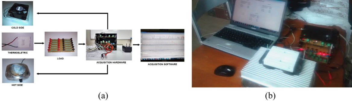
Fig. 11. Diagram system mounting blocks (a) and assembled experiment (b).
