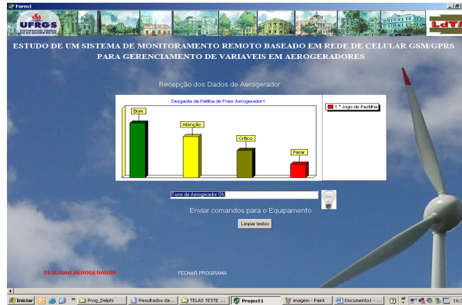
Figure 8 – Screen wear of brake pad, option STOP LEVEL
