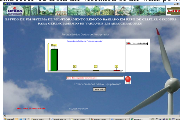
Figure 7 – Screen wind power receiving data with vibration (light red), appearing for the operator concerning simulation of vibration of the tower wind power.
